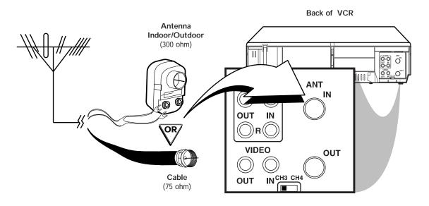
Connect the supplied black RF coaxial cable to the OUT Jack on the back of the VCR and to the ANTENNA IN Jack on the TV. (You may use either a snap-on type (supplied) or screw-on type of coaxial cable, whichever you prefer.)
